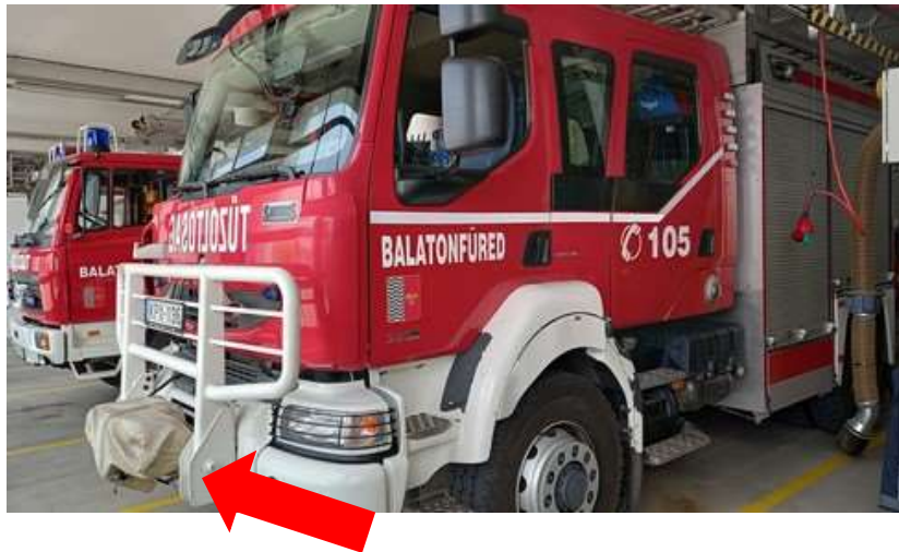
Figure 2 – Another Hungarian fire trucks and the winch. Source: [8].
