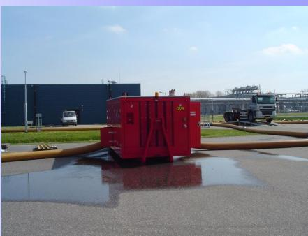
Due to sophisticated CanBus controls very easy to deploy as a BoostPump.
