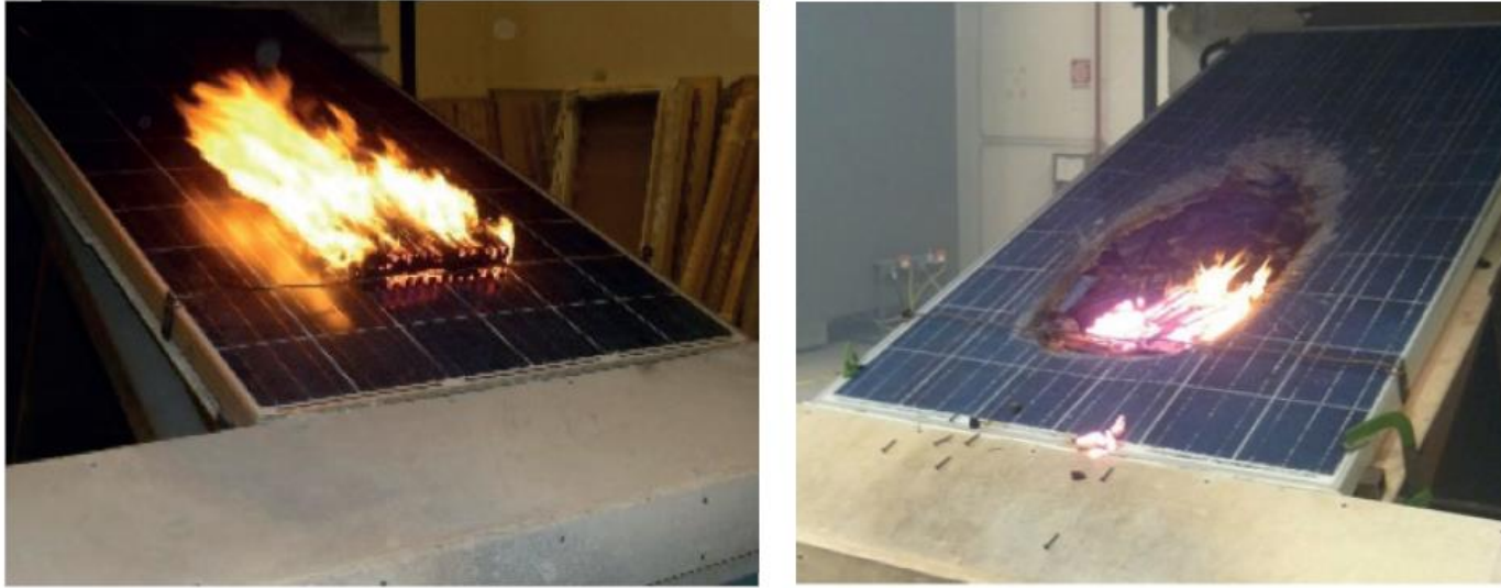
Figure 3– Example of a Class A burning-brand test – the PV module fails the test (LAPI laboratory)
